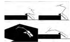
Simulation of robot climbing obstacles
