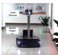
Automatic scan planning and construction progress monitoring system
