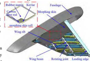
The variable-sweep morphing wing model
