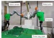
A robotic manipulation system for the cable
