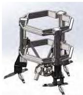
Multi-DOF adsorption type parallel mechanism
